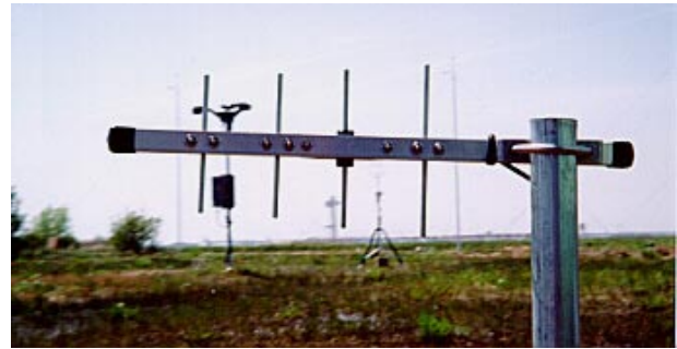
Figure 3. Yagi Directional Antenna Used To Monitor Approaches to One Runway
